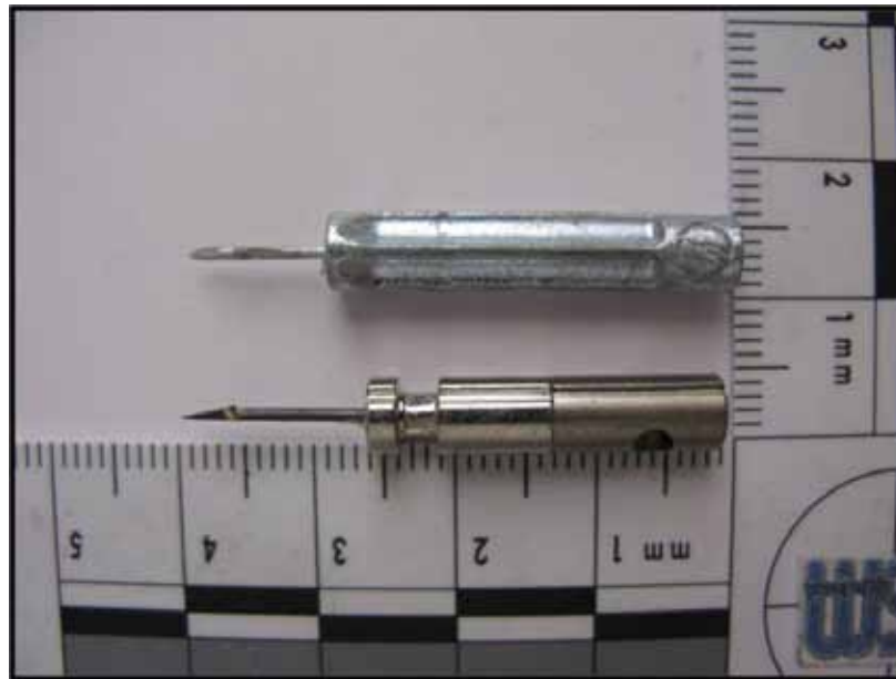
Figure 5a: The new X3 model probe (Top) vs. the X26, M26, & C2 (Bottom)
